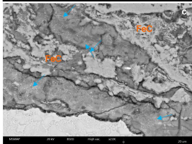
*The presence of manganese sulphide inclusions could be considered as problematic referring to the modern use of this metal in steel desulfurization processes, but the use of manganese (magnesia nigra) to prepare crucible steel is recommended in Arabic written documents from the 11<sup>th</sup> century (3).*
